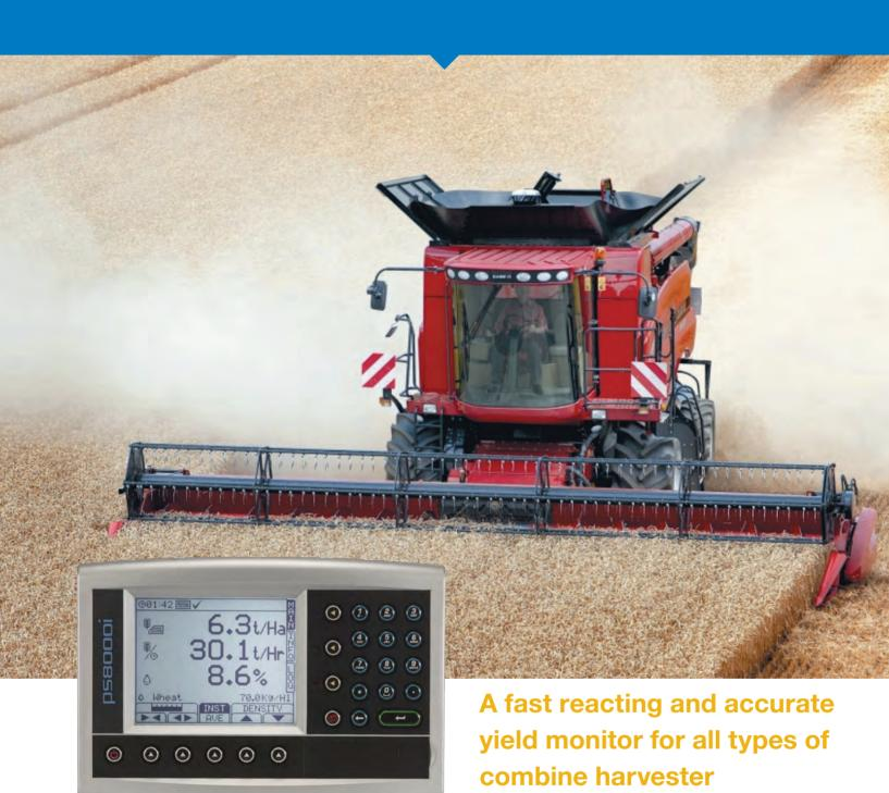
The RDS *Ceres 8000i* uses 'state of the art' optical sensing technology to measure live yield and displays dry/wet harvested weight. Now with integral SD card reader for straight forward transfer of data to a PC.
